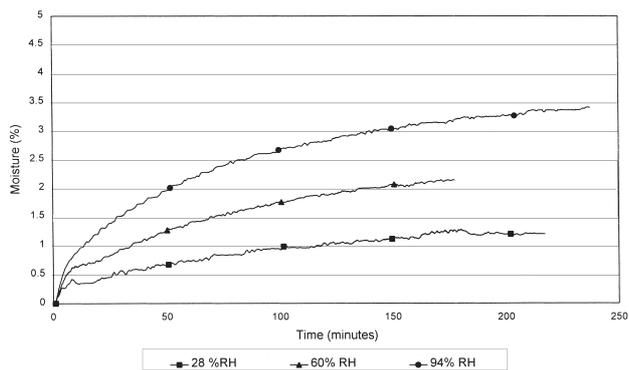
Figure 4—Moisture uptake rates for thermally dried coal from Bank Colliery at different relative humidities
