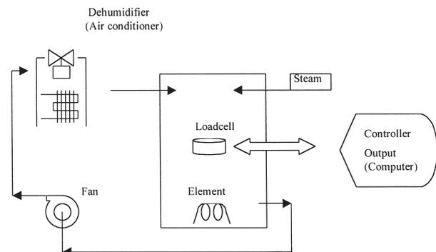
Figure 2—Diagram of experimental set-up (climate box)
