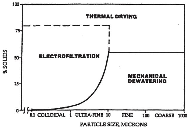
Figure 1—Effective dewatering techniques in relation to particle size<sup>4</sup>
