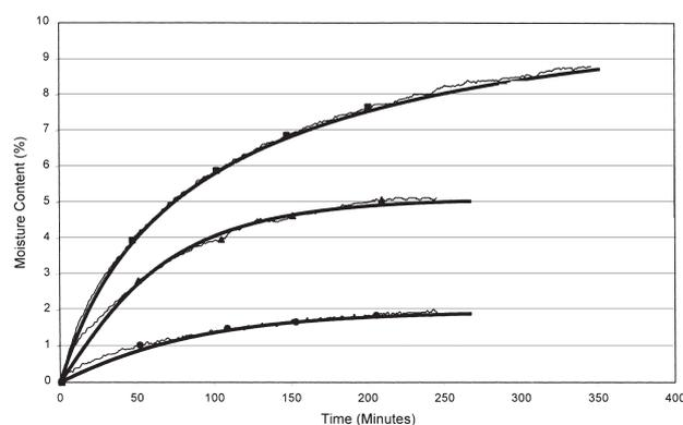
Figure 7—Model compared to experimental data for thermally dried Sigma coal
