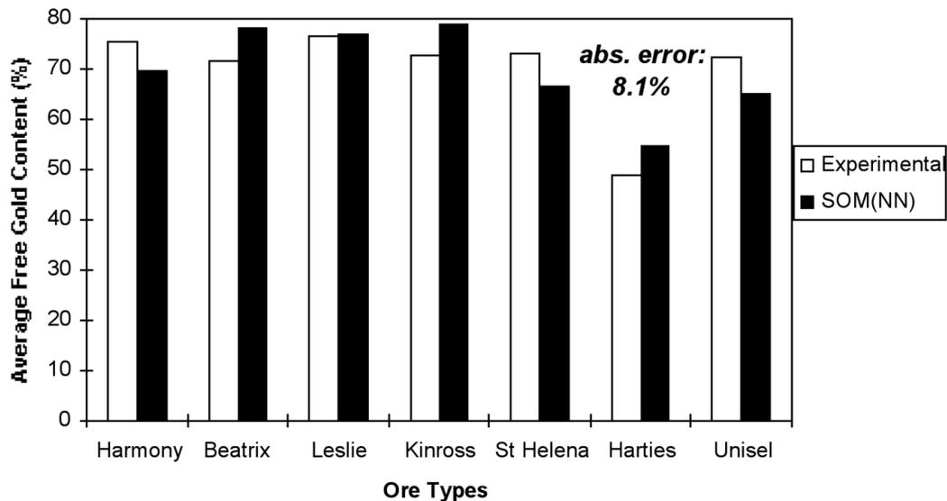
Figure 5—Neural net prediction of the average free gold (milled) for each ore type. Absolute error: 8.1%. The major contributor to error is due to poor prediction of +300  $\mu\text{m}$  size fraction
