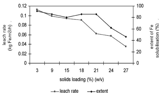
Figure 2—Bioleach rate and extent of iron solubilization as a function of total solids loading (comprised of 3% pyrite, the remainder quartz)
