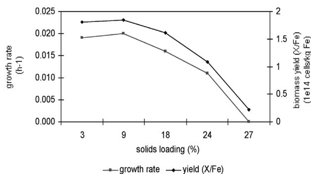
Figure 4—Microbial growth rate and biomass yield ( $Y_{X/Fe}$ ) in terms of microbial cells produced per kg iron oxidized as a function of total solids loading (comprised of 3% pyrite, the remainder quartz)
