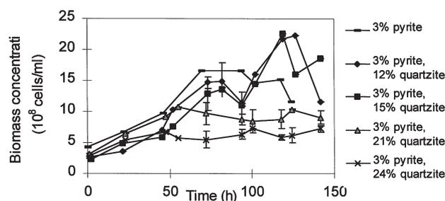
Figure 3—Effect of solids loading on the growth rate of *Sulfolobus metallicus* on exposure to 3% pyrite and 0 to 24% inert quartzite
