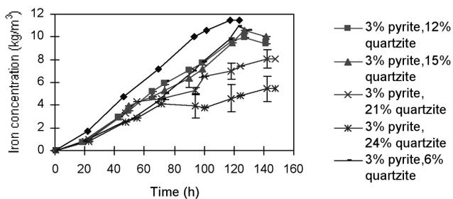
Figure 1—Effect of solids loading on the rate of iron leaching of pyrite in the presence of *Sulfolobus metallicus* on exposure to 3% pyrite and 0 to 24% inert quartzite
