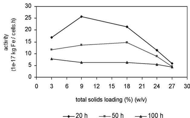
Figure 5—Microbial cell activity in terms of specific pyrite oxidation rate as a function of solids loading and duration of experiment
