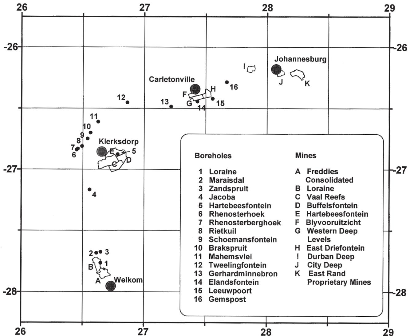
Figure 1—Locality map of Witwatersrand gold mining areas showing positions of boreholes (1–16) and mines (A–K) from which rock samples analysed for thermal conductivity, density and heat capacity were derived. Boreholes are named after farms on which they were drilled
