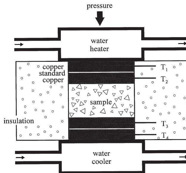
Figure 3—Cross-section of the divided-bar apparatus for measuring thermal conductivity.  $T_1$  to  $T_4$  represent thermistors inserted into holes drilled radially to the centres of the copper discs
