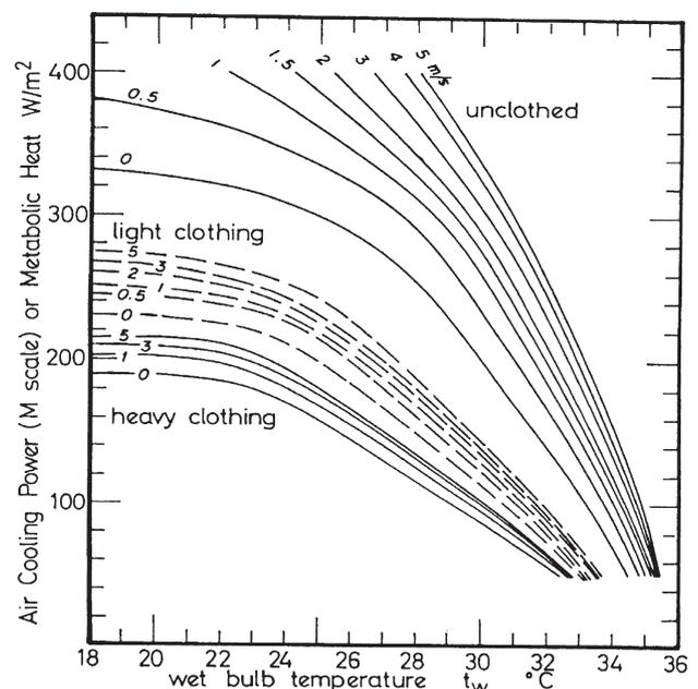
Figure 1—Air Cooling Power (M scale) or ACPM (after McPherson<sup>8</sup>)
