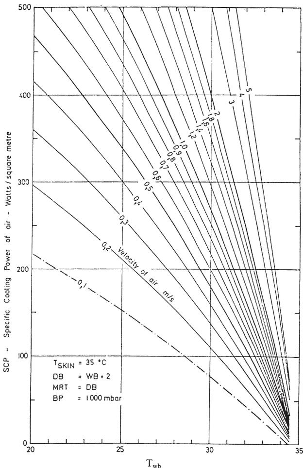
Figure 2—SCP values for various air velocities (after Dumka<sup>9</sup>)
