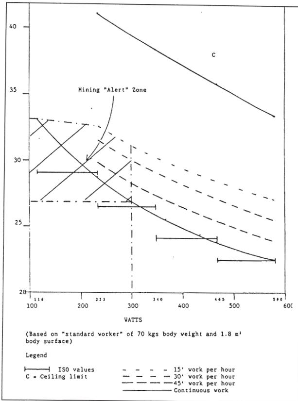
Figure 3—NIOSH and ISO heat stress limits for acclimatized mineworkers in terms of WBGT and metabolic heat load (after Graveling *et al.*<sup>20</sup>)
