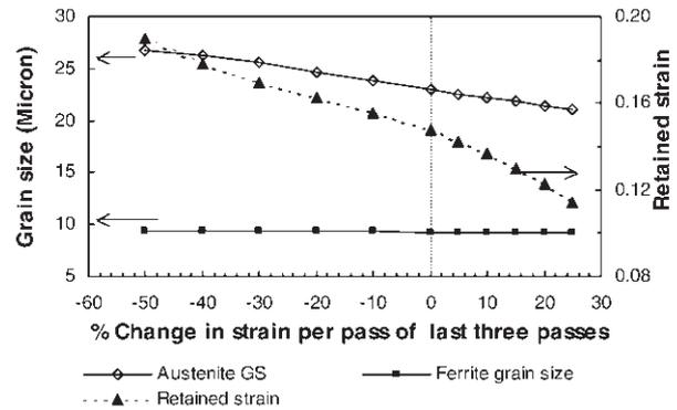
Figure 10—Sensitivity analysis of changing the reductions per pass of the three last passes (F3 to F5) by an equal percentage and transferring these changes evenly to the remaining first four passes (R1 to F2) to maintain a constant total reduction from the 75 mm slab to a 2 mm strip
