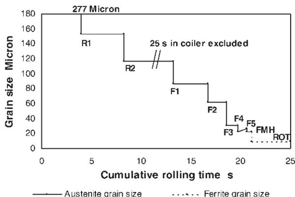
Figure 8—Austenite grain size development (R1 to FMH) shown for a 75 mm slab reduction to 2 mm hot rolled strip as well as the calculated final ferrite grain size (FMH to ROT) expected in the strip. FMH = Finishing Mill Head, and ROT = Run-out Table. Note that 25 seconds from the transfer bar's temperature equalization time in the coil box have been excluded from the accumulated time
