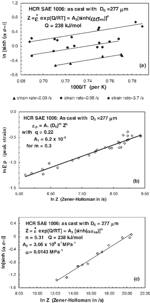
Figure 5—Hot deformation curves for the HCR as-cast coarse grained SAE 1006 steel with the curve (a) used to find the activation energy  $Q$  from Equation [1], (b) used to find the values for  $q$  and  $A_1$  from Equation [2] and (c) the overall hot deformation curve combining all of the data in terms of Equation [1]. Line fitting: regression coefficients  $R^2$  were larger than 0.950 in all cases except for the top line in Figure (a) where  $R^2 = 0.905$
