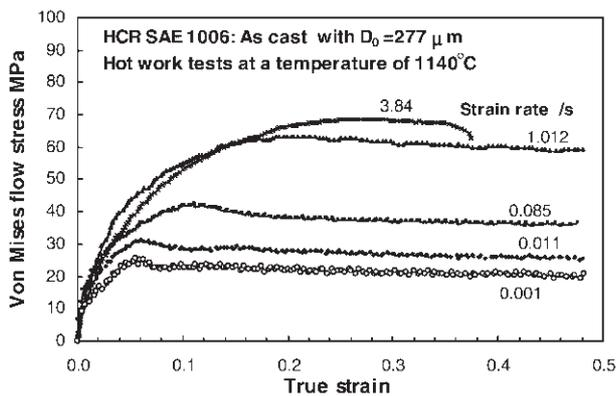
Figure 3—High temperature flow stress curves of as-cast HCR-processed SAE 1006 steel, tested at 1140°C at different strain rates
