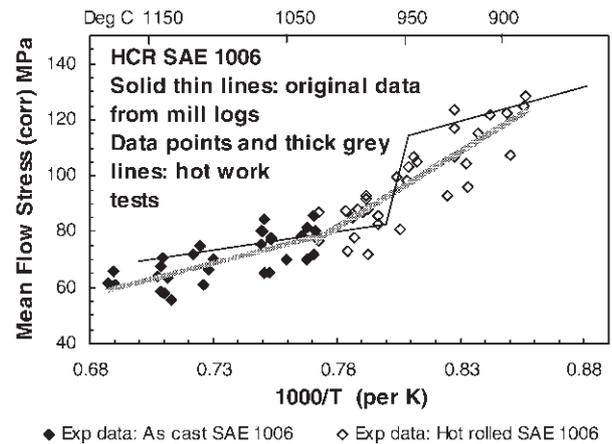
Figure 4—Mean Flow Stress values determined from hot deformation tests and plotted on the mill log derived lines from Figure 3 for both the HCR as-cast coarse grained material (filled symbols) and the finer grained hot rolled material (open symbols)
