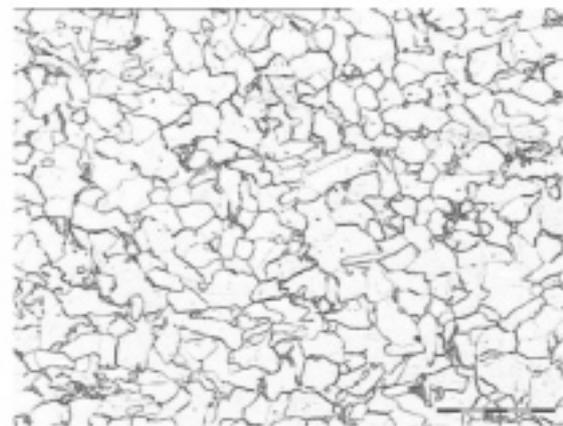
Figure 7—The non-uniform ferrite grain size distribution of the plant produced HCR-slab analysed in Table IV. Etchant used: 2% Nital. (Micrograph kindly provided by Verdoorn<sup>34</sup>.)
