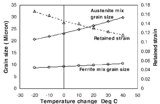
Figure 9—Sensitivity effects on the predicted austenite grain size at the FMH, on the predicted ferrite grain size after the FMH, and on the retained strain in the austenite just before transformation to ferrite, are shown as a function of changing the product/process temperatures along the entire line by a set amount
