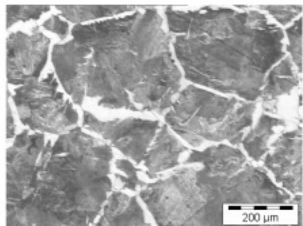
Figure 2—Prior austenite grain size structure at 1200°C of the SAE 1006 low carbon steel processed by the HCR-route and in the as-cast condition. The prior austenite grain boundaries at 1200°C have been decorated by cementite through hyper-eutectoid carburization. Etchant used: 2% Nital
