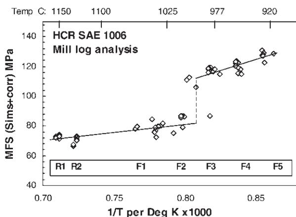
Figure 1—The Mean Flow Stress (in MPa) from mill logs as a function of the reciprocal absolute temperature  $1/T$  (in  $\text{K}^{-1}$ ) of the low carbon steel SAE 1006 and processed by the HCR-route
