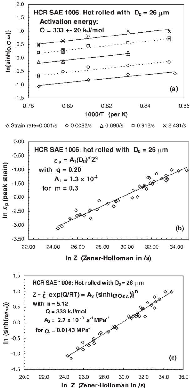
Figure 6—Hot deformation curves for the HCR hot rolled and fine grained SAE 1006 steel with the curve (a) used to find the activation energy  $Q$  from Equation [1], (b) used to find the values for  $q$  and  $A_1$  from Equation [2] and (c) the overall hot deformation curve combining all of the data in terms of Equation [1]. Line fitting: regression coefficients  $R^2$  were larger than 0.950 in all cases
