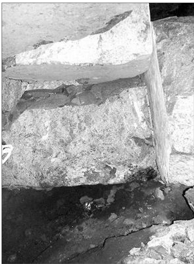
Figure 5—Photograph showing a FOG that occurred due to low confinement conditions
