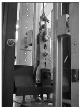
Figure 6—Mechanism for early detaching, with striking pin
