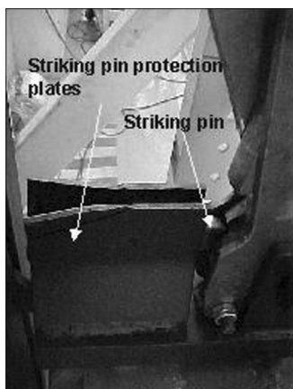
Figure 7—Mechanism for early detaching, with striking pin and protection plates
