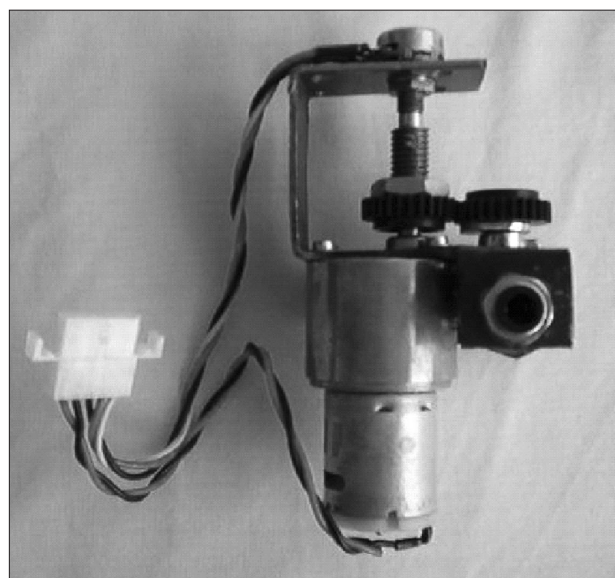
Figure 2—Standard irrigation ball valve operated by a geared motor
