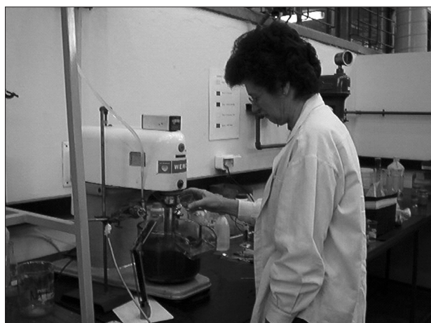
Figure 1—Arrangement of flotation test cell
