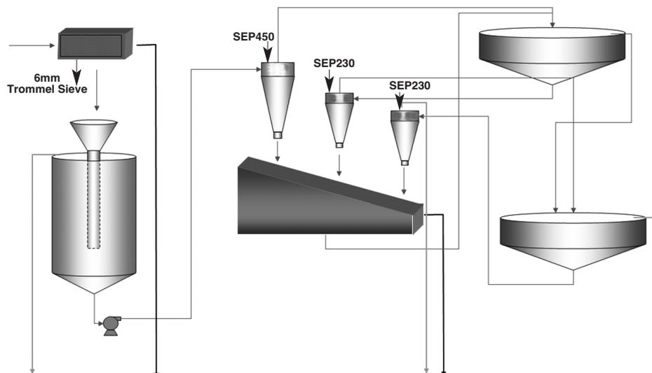
Figure 1—Current process flow diagram for gypsum recovery at Afmine
