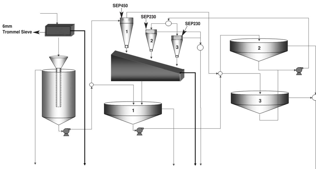
Figure 4—Alternative process flow diagram for gypsum recovery at Afmine
