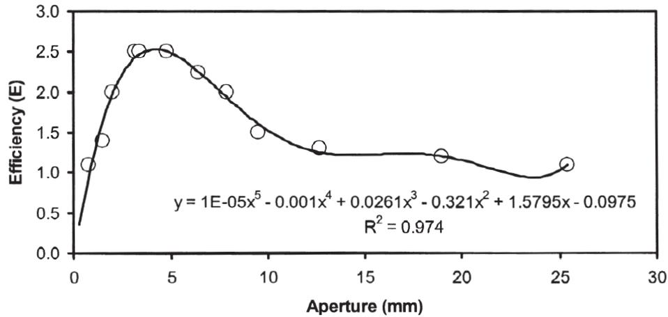
Figure 2—Estimation of the efficiency for the linear screen
