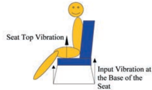
Figure 2—Person on seat with input vibration at the base of the seat and measured response at the seat top
