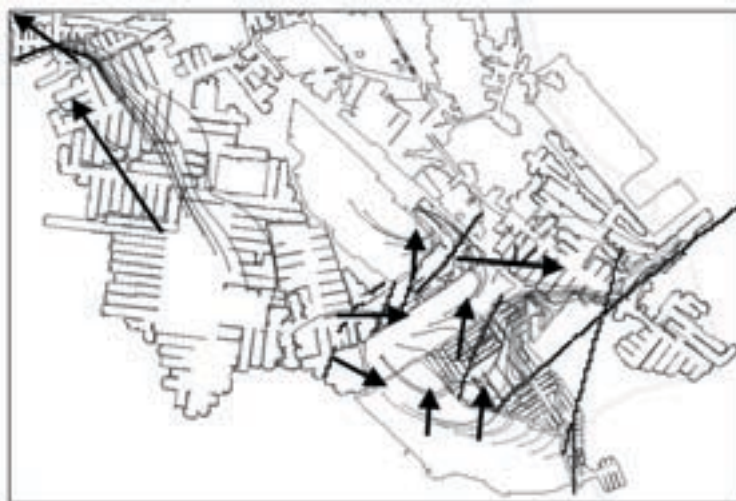
Figure 5—Identification of groundwater flow paths by making us of particle tracking
