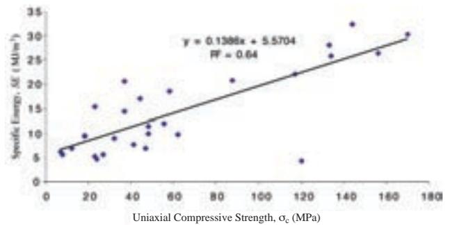
Figure 5—Relation between  $\sigma_c$  and SE for all tested rock types
