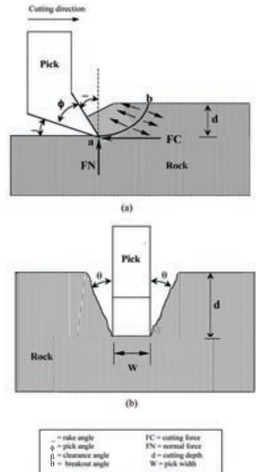
Figure 2—Tensile breakage model of Evans (a), simplified groove geometry (b)
