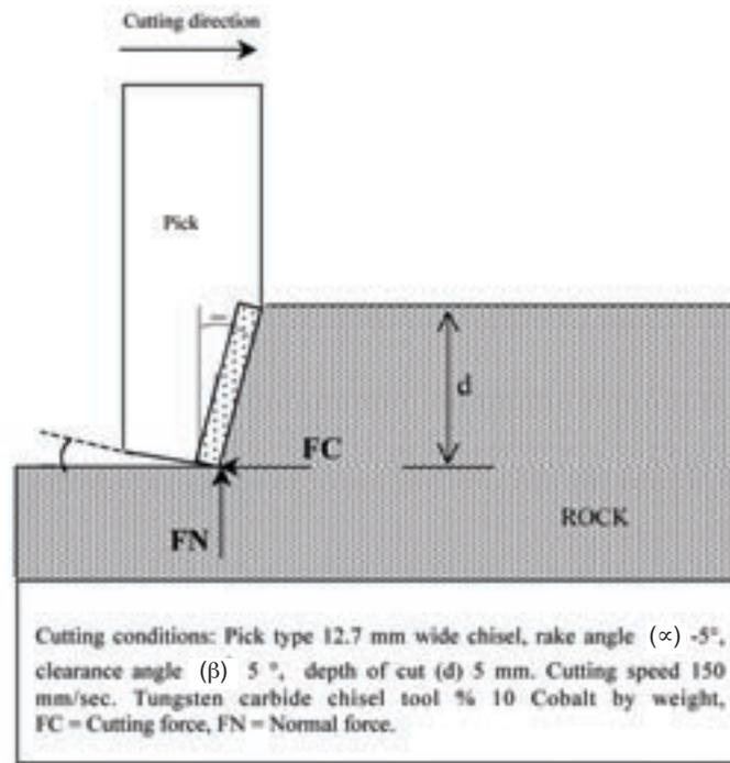
Figure 3—Details of standard laboratory cutting conditions
