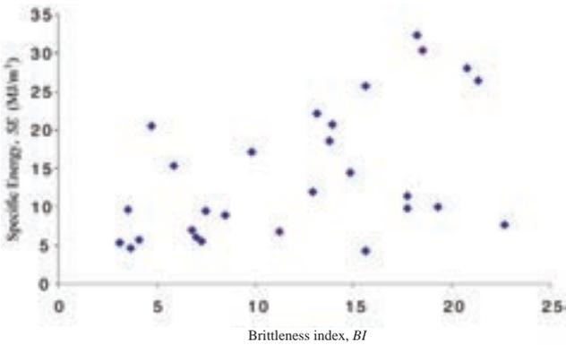
Figure 4—Relation between BI and SE for all tested rock types
