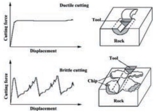
Figure 1—Brittle and ductile mode of cutting<sup>30</sup>
