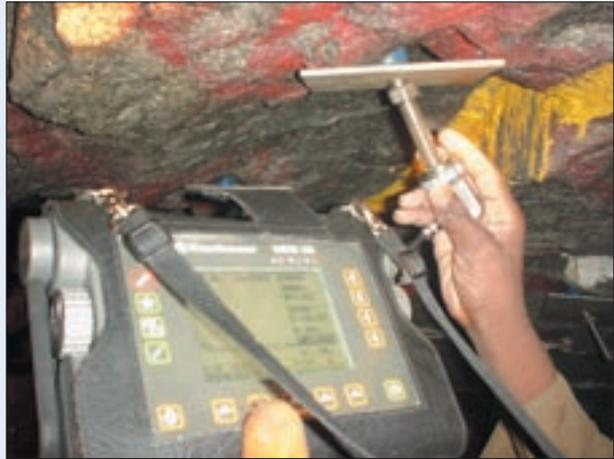
The Smartbolt is interrogated with a portable ultrasonic USM 25 DAC device, which measures the longitudinal sound velocity to assess any structural change. The probe is applied to the head of the Smartbolt and the sound velocity feedback is used to assess microstructural changes that have occurred in the roof bolt as a result of the stress exerted on it
