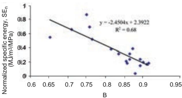
Figure 9—Relation between B and  $SE_n$  for arenaceous rocks
