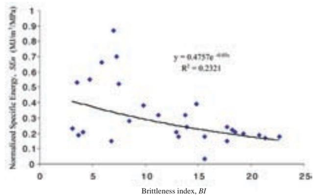
Figure 6—Relation between BI and  $SE_n$  for all tested rock types
