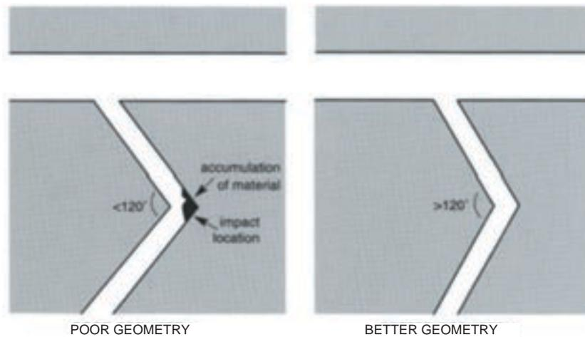
Figure 11—Effect of pass system geometry
