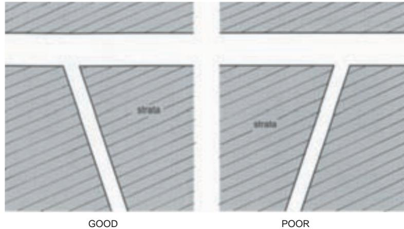
Figure 8—Preferred orientation of pass relative to the strata dip
