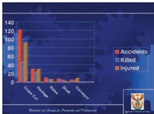
Figure 6—Locations of rockpass engulfing accidents (source B.J. Erasmus, DME)
