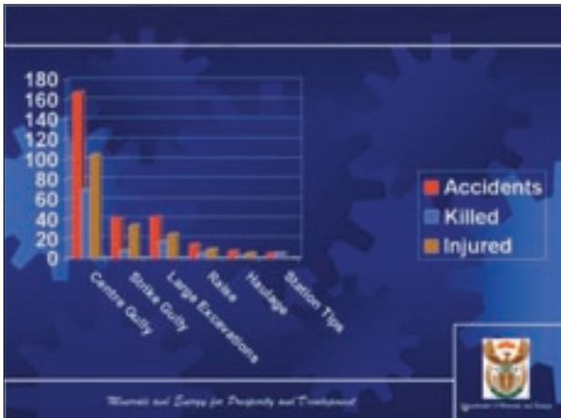
Figure 2—Locations of accidents: falling into rockpasses (source B.J. Erasmus, DME)
