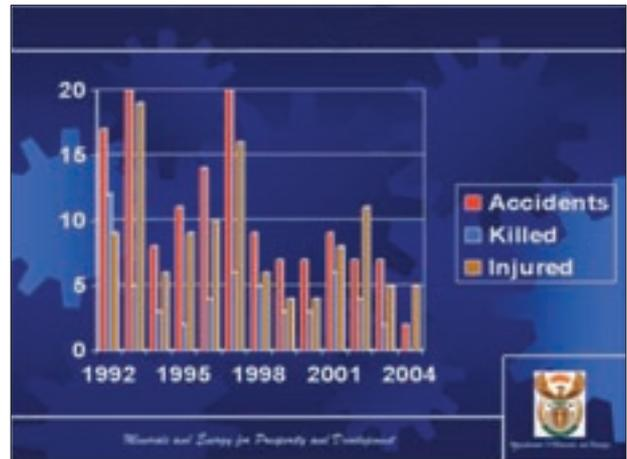
Figure 5—Accident record: engulfed by material from rockpass (source B.J. Erasmus, DME)
