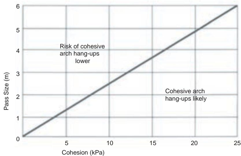
Figure 10—Guideline pass size with regard to 'sticky' material
