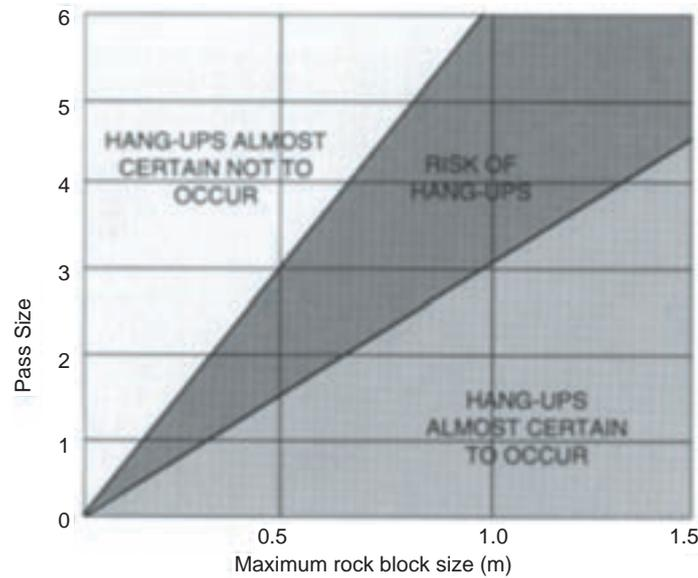
Figure 9—Indication of pass size relative to rock fragment size
