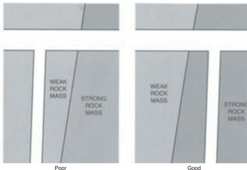
Figure 7—Recommended location of pass with respect to rock quality
