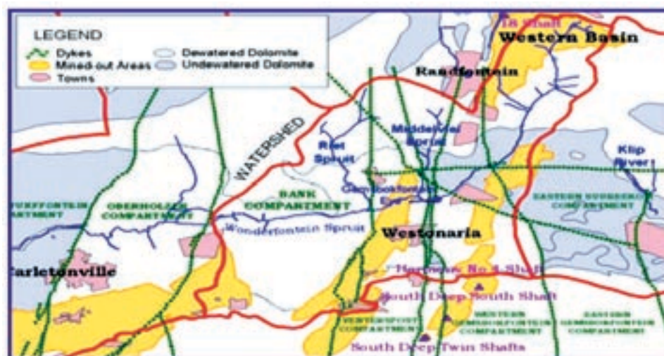
Figure 5—The dolomitic compartments (source: South African Mining World , September, 1982)
