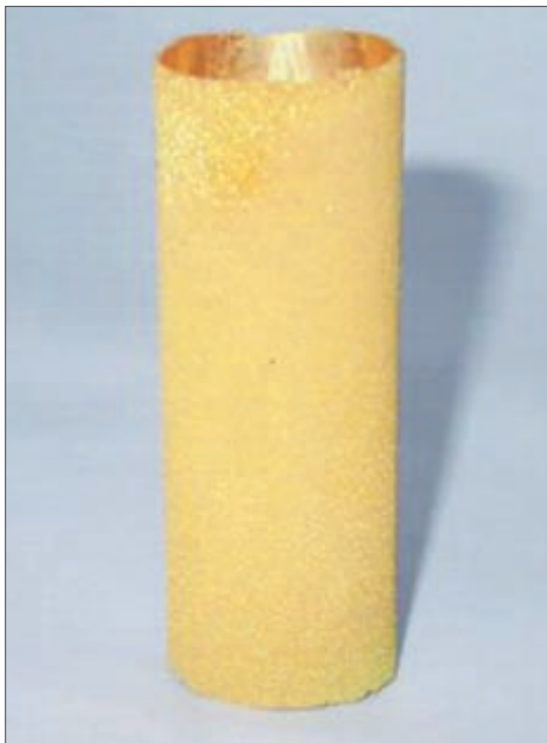
Figure 7—Electroformed tapered tube of gold/silver alloy produced in the EWEF Mark I cell
