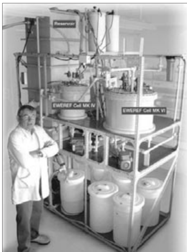
Figure 8—Small-scale gold recovery pilot plant, showing the 400 l reservoir and the EWEREF Mark IV and Mark VI cells
