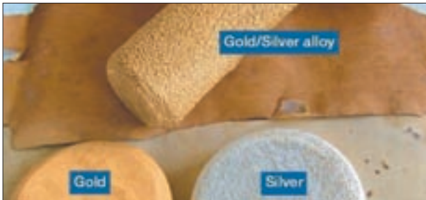
Figure 9—Gold, silver and gold/silver alloy electroforms produced in the EWEF Mark IV cell
