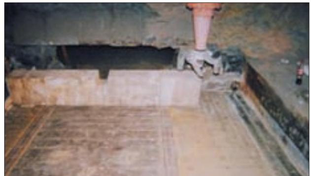
Figure 5—SAVELINE sensors applied in the condenser floor of an Imperial Smelter
