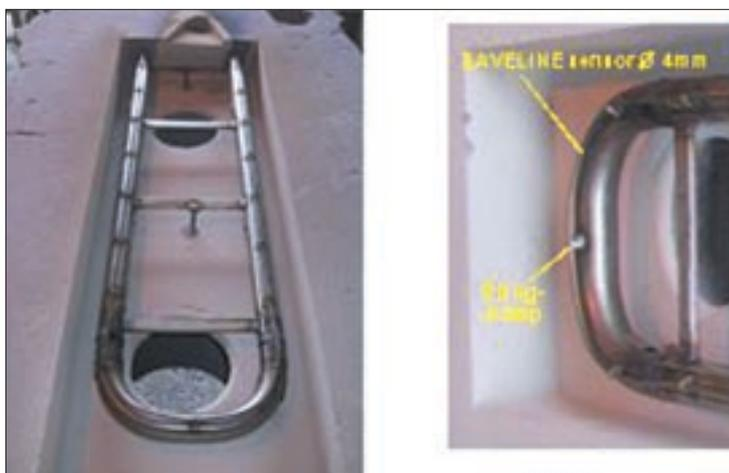
Figure 8—Prepared metal tube inside the sand mould
