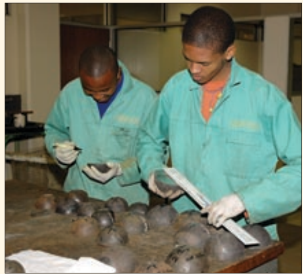
Quality control work on sectioned grinding ball in Mintek's metallographic laboratory
