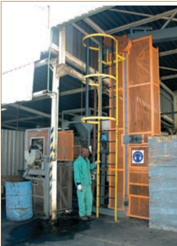
A drop tester (right) and grinding ball mill used at Mintek for impact and wear tests
