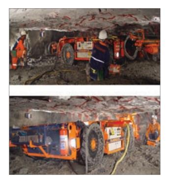
SMC MKII drill rig and roofbolter at Waterval
