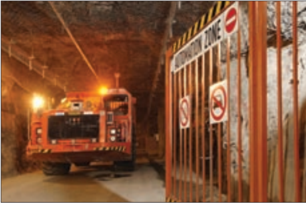
Figure 4—Toro 50D dump truck at ACS gate
