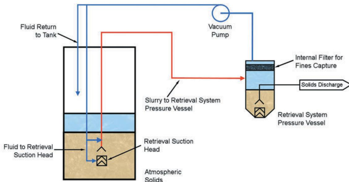
Figure 2—AtmoTrans retrieval operation
