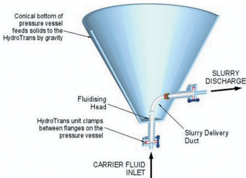
Figure 1—HydroTrans installation on a pressure vessel
