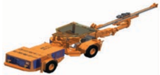
Figure 14—Axess rig for gully development
