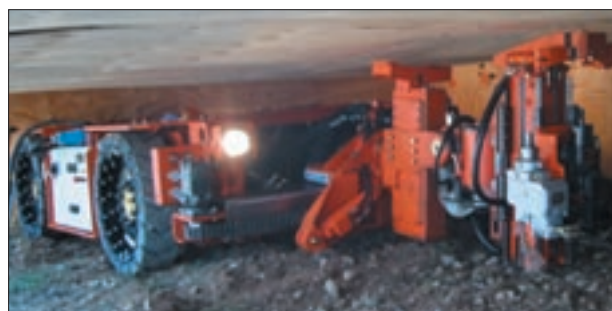
Figure 9—Roofbolter in a mock-up stope 1.1 metres high
