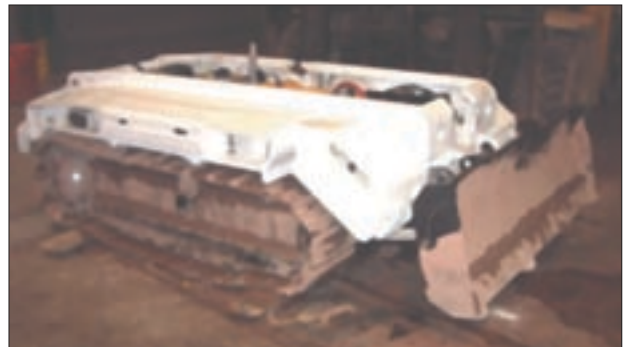
Figure 15—Remotely operated bulldozer
