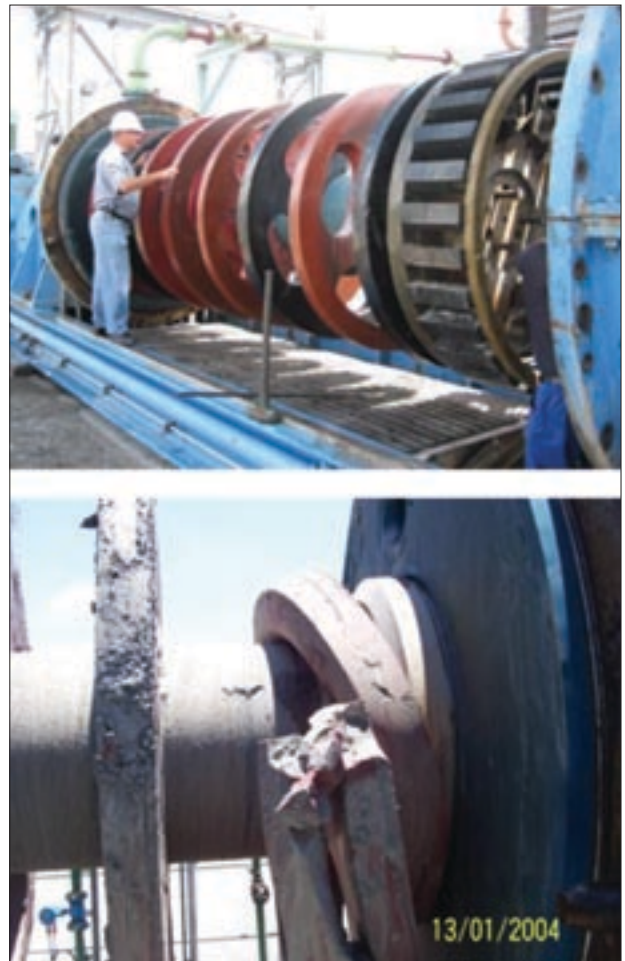
Figure 10—Photographs of the M 10 000 mill internals, showing the damaged discs and the discs after replacement following one of the internal failure incidents
