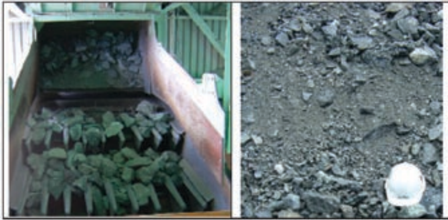
Figure 6—Photos illustrating poor (left) and good fragmentation (right). The impact of the poor fragmentation (choking the grizzly) is evident in the left photo
