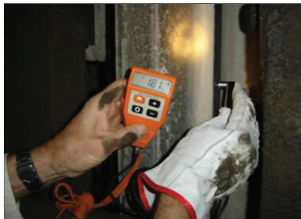
Figure 8—Another shaft guide. This measuring taken on the side gives 181 \mu\text{m} of hot dip galvanized coating
