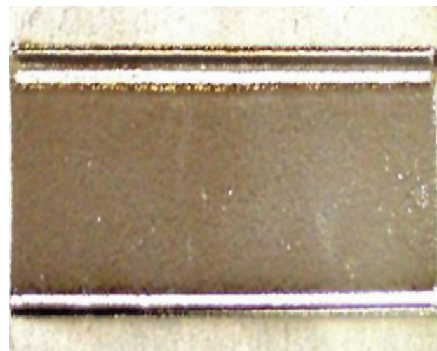
Figure 3—Laser processed surface under argon atmosphere
