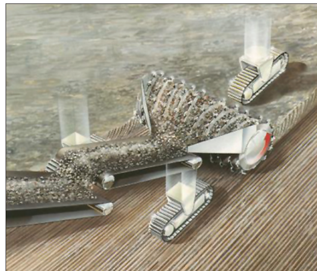
Figure 3—Operational system of Wirtgen surface miner 13
