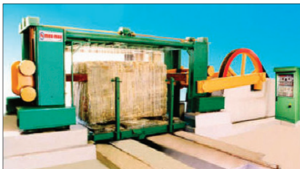
Figure 2—Gang saw during the cutting
