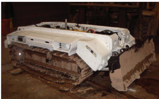
Figure 6—Remotely operated bulldozer
