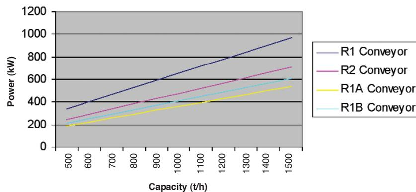
Figure 5—Motor power requirements
