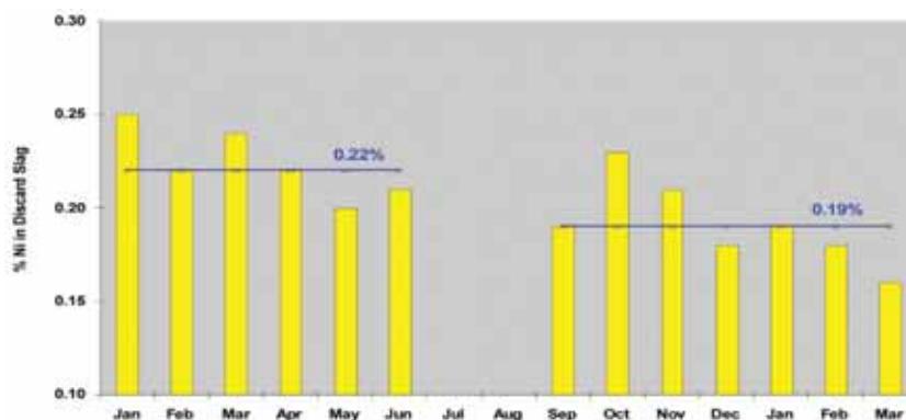
Figure 9—Improvement in discard Nickel slag losses
