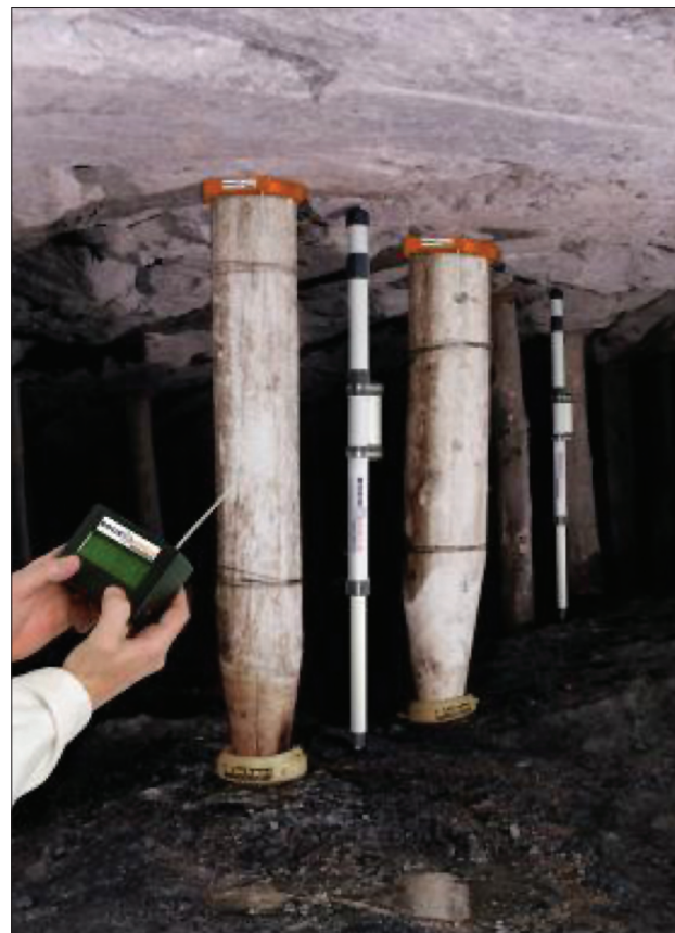
Figure 4—Continuous closure logger used to measure panel closure (hand-held radio communication unit also shown)
