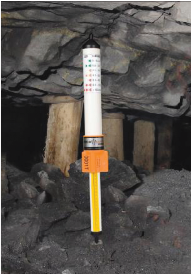
Figure 11—A photograph of the Closure Telltale
