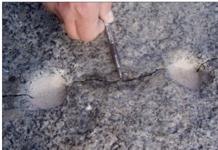
Figure 1—Rock fracture between two neighboring holes by the NEEM in a granite mine (Arshadnejad, 2010)
