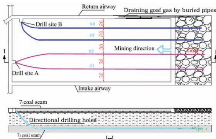
Figure 9—Schematic of gas drainage
