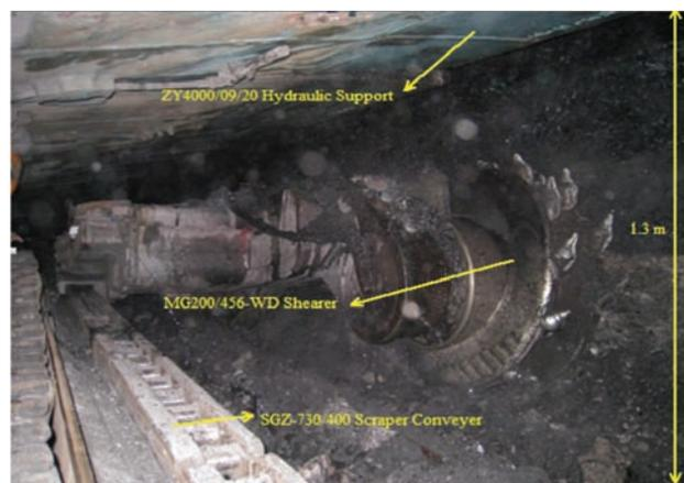
Figure 7—The longwall equipment in Qinan Coal Mine
