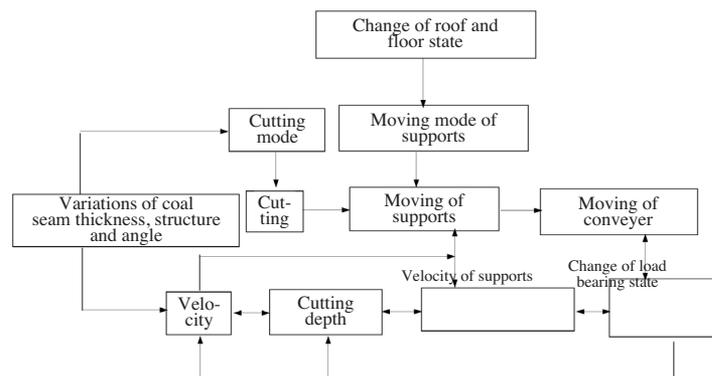
Figure 1—Intelligent control system of highly mechanized workforce
