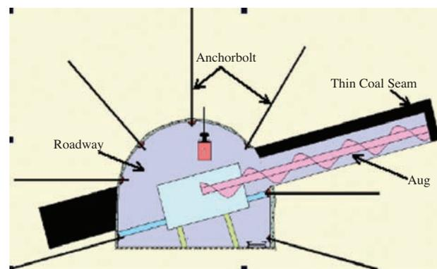
Figure 2—Working layout of auger in the roadway
