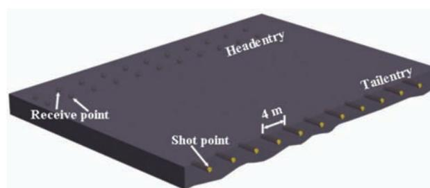
Figure 3—Schematic of the seismic monitoring system
