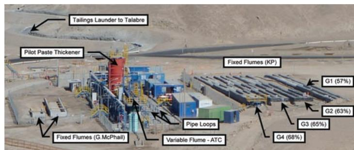
Figure 1—Pilot plant layout
