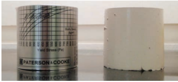
Figure 6—Boger slump of kaolin paste with a Bingham yield stress of 1 120 Pa
