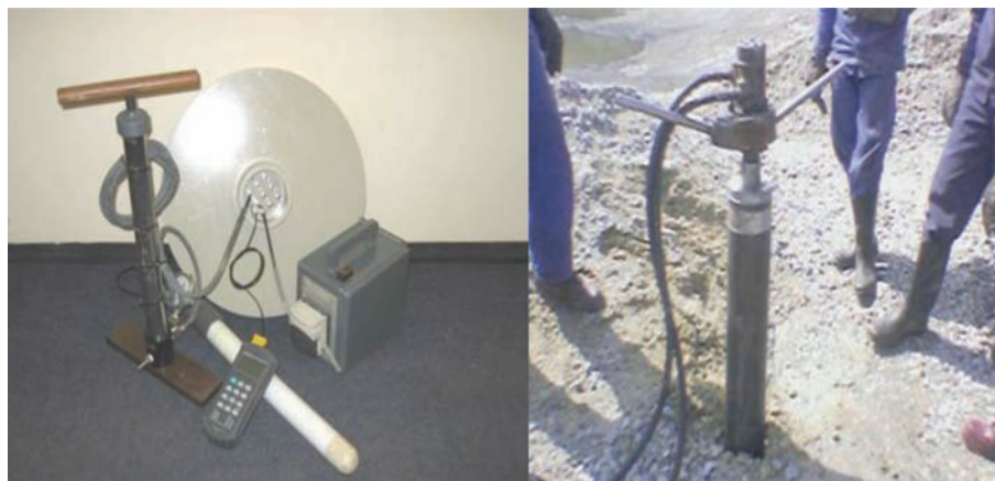
Figure 11—In-heap monitoring probes and auger
