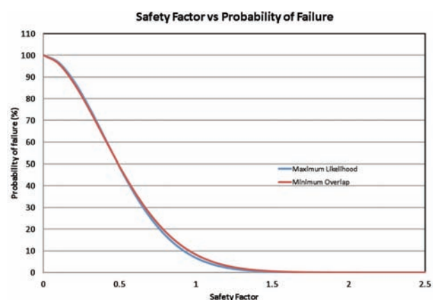
Figure 7 – Comparison between probabilities of failure and safety factors obtained by using the maximum likelihood and overlap reduction methods. The curves were obtained by extrapolation for the range of safety factors less than 0.7
