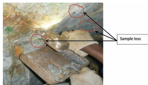
Figure 12—Sample loss clearly visible when the chipper is using a hammer to collect sample
