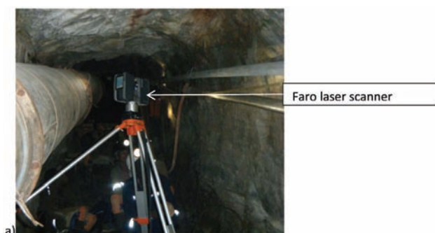
Figure 5—Faro laser scanner used to measure the actual volume and three-dimensional shape of material removed during the chipping process
