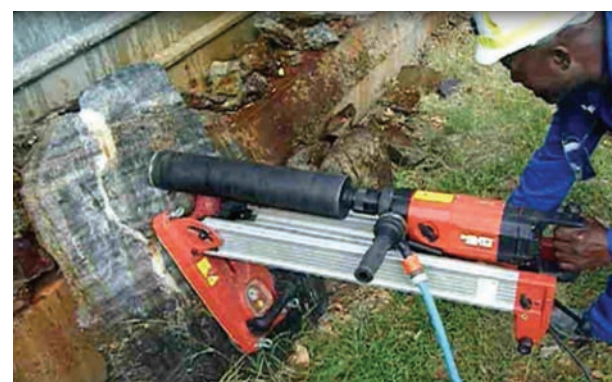
Figure 8—Drilling core samples from reef material on surface was successful and promising. It was possible to extract a 15 cm length of core in less than 15 minutes
