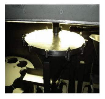
Figure 8-Airtight lid to prevent any dust loss/ingress
