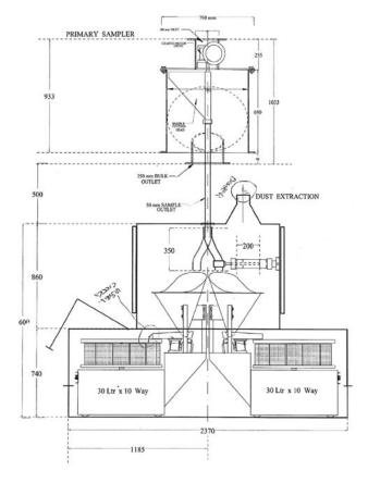
Figure 1—Schematic design of Vezin sampler and the two rotary splitters used to collect the interleaved increments from the Vezin
