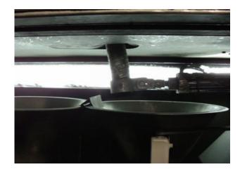
Figure 3–Oscillator to direct a flexible tube channelling the sample into the respective hoppers
