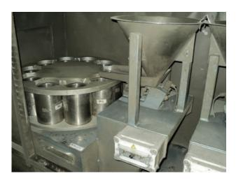
Figure 4-10-way splitter used for the sub-sampling of the interleaved samples
