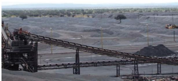
Figure 9—Numbered and sampled manganese stockpiles ready for blending
