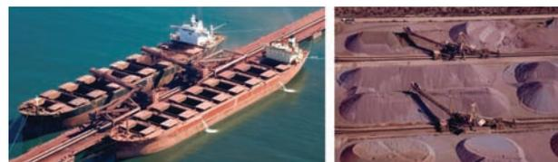
Figure 12—(a) Dual shiploaders at the Saldanha port loading facility, and (b) stacker-reclaimers in the stockpile area at the Saldanha port loading facility (source: Kumba Iron Ore, 2010)
