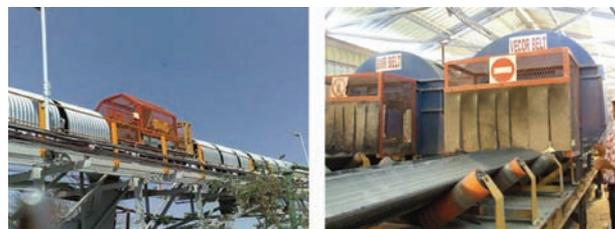
Figure 3—Go-belt sampler installation on conveyor belts from shaft head (source: Letsie, 2009; Minnitt, 2013)
