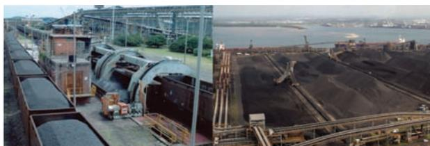
Figure 13—(a) Coal tipplers transferring coal at Richards Bay before (b) being stacked on blending stockpiles
