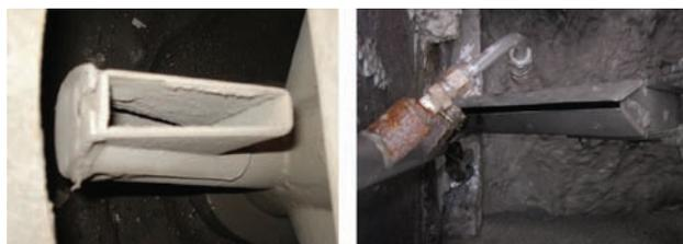
Figure 5—(a) Vezin sampler splits the primary residue sample, and (b) cleaning nozzle pointing at head grade sampling by cross-stream cutter (source: Kelly, 2007)
