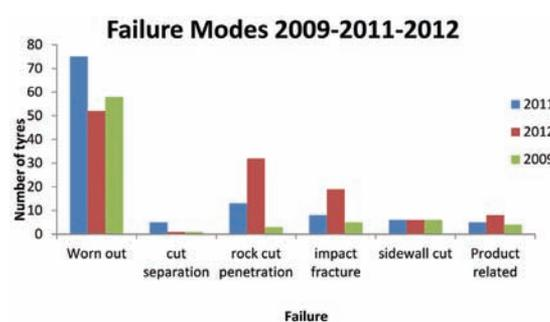
Figure 4—Failure modes
