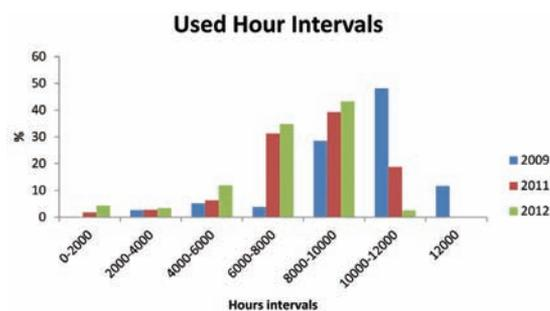
Figure 3—Frequency graph for average tyre hours
