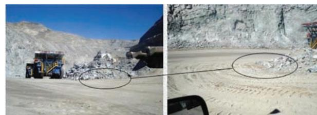
Figure 6—An example of loose rocks in a turn, with a truck about to cut a corner
