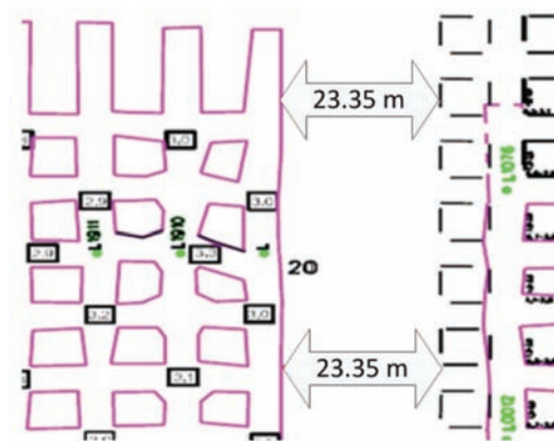
Figure 1—Mining layout showing barrier pillars
