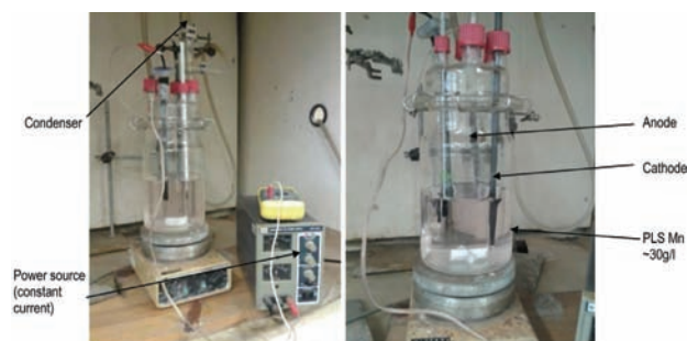
Figure 2—Experimental set-up for the production of EMD
