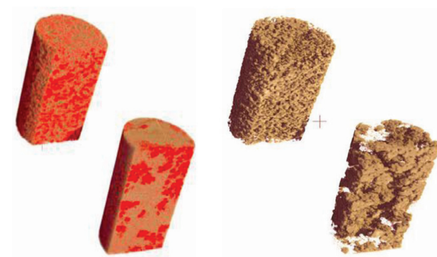
Figure 5 – Left: the grouped pyroxene mineral (coloured red) can be clearly seen in norite (top), and different concentration of feldspar are observed in anorthosite (bottom) in a thin slice. Right: transparent corresponding neutron tomograms. The minerals shown are only pyroxenes that are present in both norite and anorthosite but at different concentrations [archives from Necsa's Nrad and MIXRAD system]
