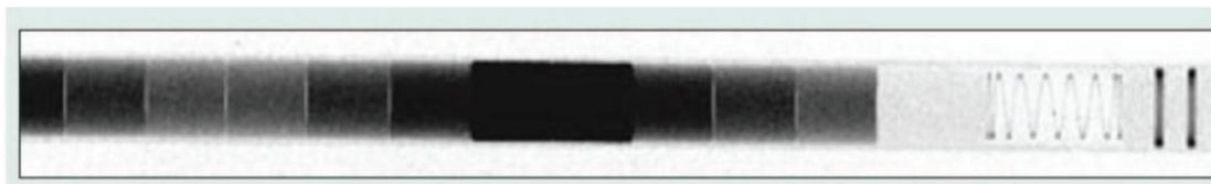
Figure 8 – Neutron radiograph (film) of fresh fuel pellets in a fuel pin with varying degrees of isotopic U-235 enrichment. Pellets with higher enrichment appear darker (Frajtag, n.d.)
