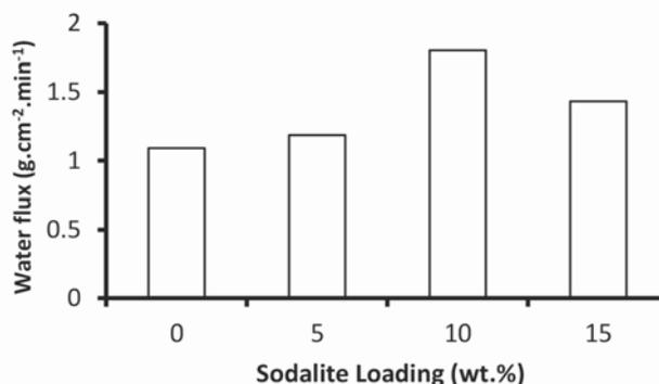
Figure 7 – Membrane flux as a function of the SOD loading. Experimental conditions: pump speed: 12 revolutions per second (flow rate); pressure: 1 atm; temperature:  $25^{\circ}\text{C}$ ; filtration mode: cross-flow
