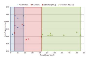
Figure 3—Matte tapping temperature vs. productivity per tap-hole. PGM and Ni smelters based on survey, selected Ni and Cu smelters based on literature data (Schlesinger et al., 2011; Davenport et al., 2003)
