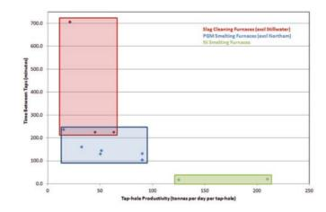
Figure 5-Time between taps vs. taphole productivity for slag cleaning furnaces, PGM smelting furnaces, and Ni smelting furnaces
