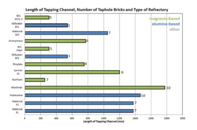
Figure 1-Length of tapping channel, number of tap-hole bricks, and type of refractory
