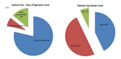
Figure 7-Tap-hole clay - type of aggregate and binder used
