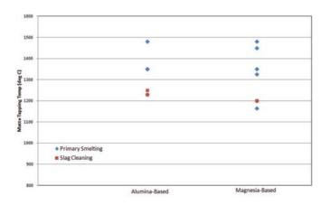
Figure 2-Matte tapping temperature vs. tap-hole brick type
