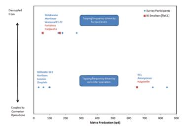
Figure 4-Level of coupling to converter operations vs. smelter matte production for survey participants and literature data (Schlesinger et al., 2011)
