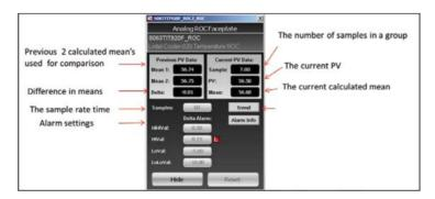
Figure 10-ROC pop-up configuration on SCADA
