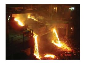
Figure 13-Draining of furnace for deep tap-block repair
