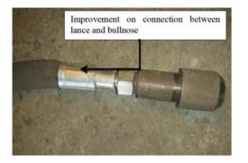
Figure 16-New bullnose design for oxygen pipe
