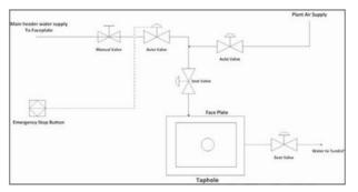
Figure 18-Emergency system for the cooling water supply
