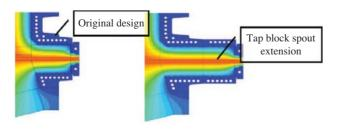
Figure 6-Extended tapping channel
