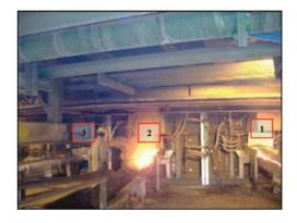
Figure 2-Slag tap-block layout
