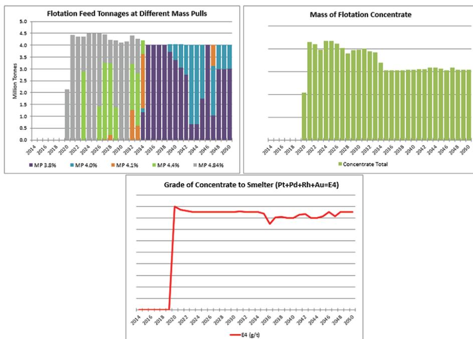
Figure 8—Optimization of mass pull to flotation concentrate
