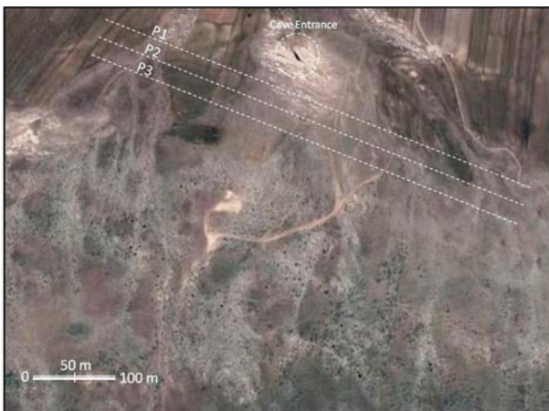
Figure 6—Aerial photograph of the studied area. The cave entrance is visible at the north of the image. The location and trend of each survey line is illustrated (image from Google Earth® software)
